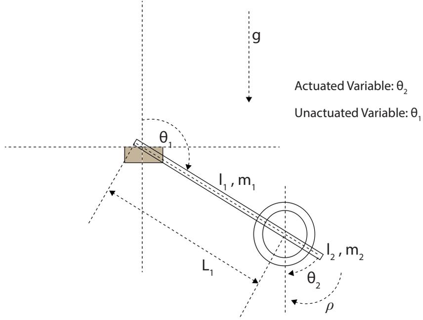
FIGURE 2.1: Schematic representation of IWP (Inertia Wheel Pendulum [15]).
