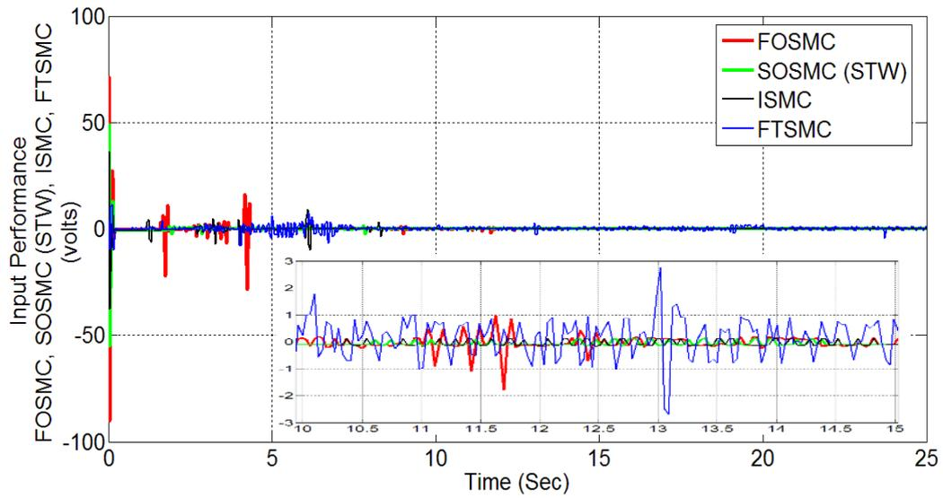
FIGURE 5.15: Control Input profile of FOSMC, SOSMC(STW), ISMC and FTSMC for reference tracking.
