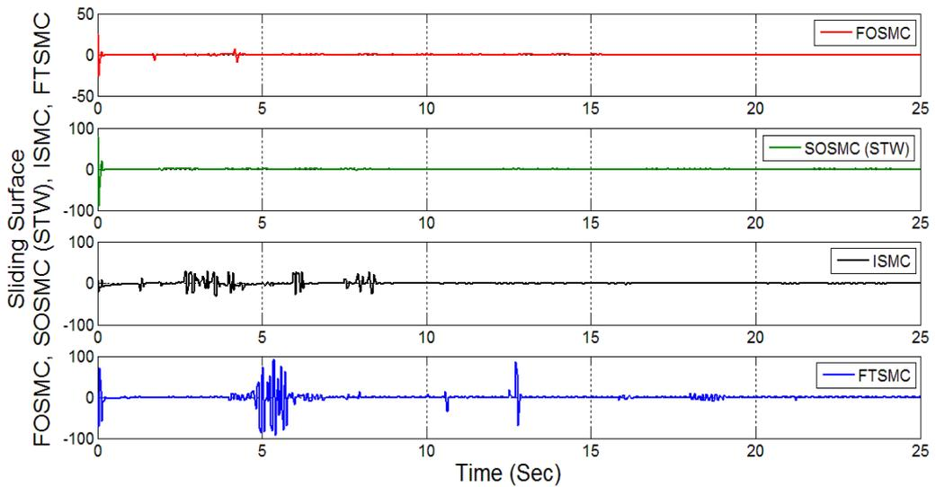
FIGURE 5.14: Separate sliding manifold convergence profile of FOSMC, SOSMC(STW), ISMC and FTSMC.
