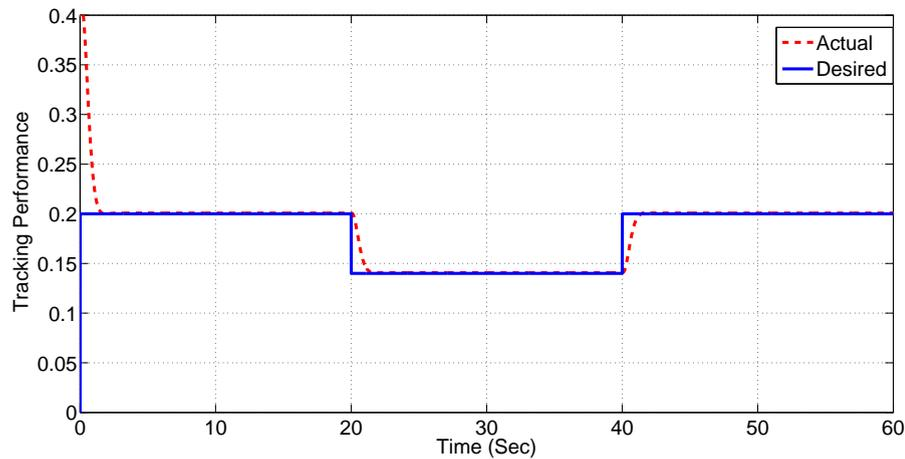
FIGURE 4.2: Output tracking performance when a square wave is used as reference/desired output.
