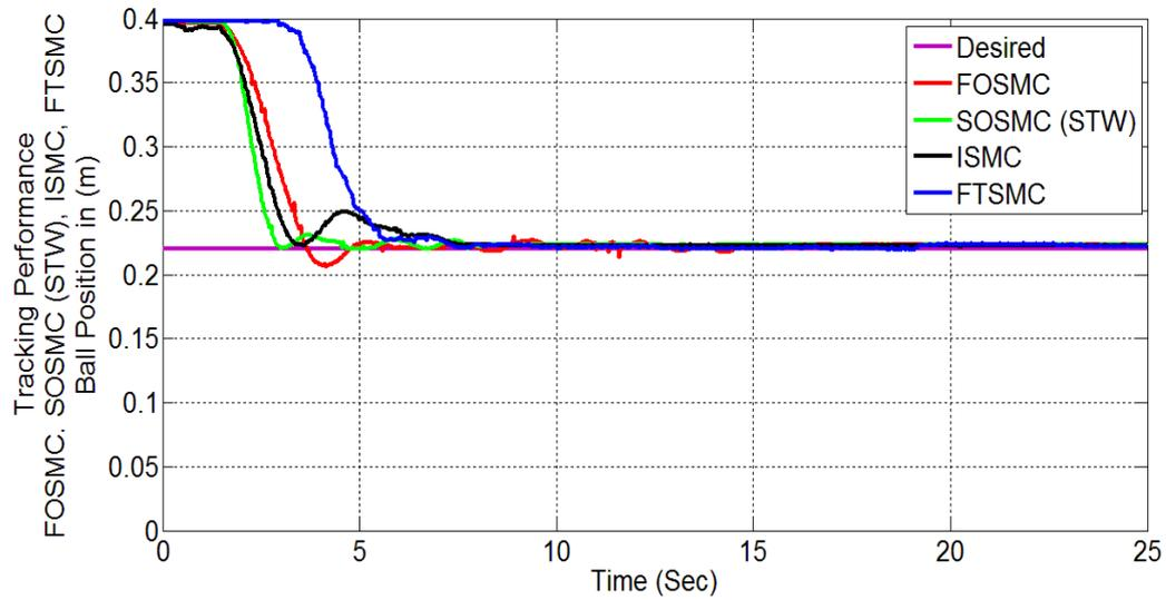
FIGURE 5.9: Output tracking performance of FOSMC, SOSMC(STW), ISMC and FTSMC,  $r_d = 22cm$ .
