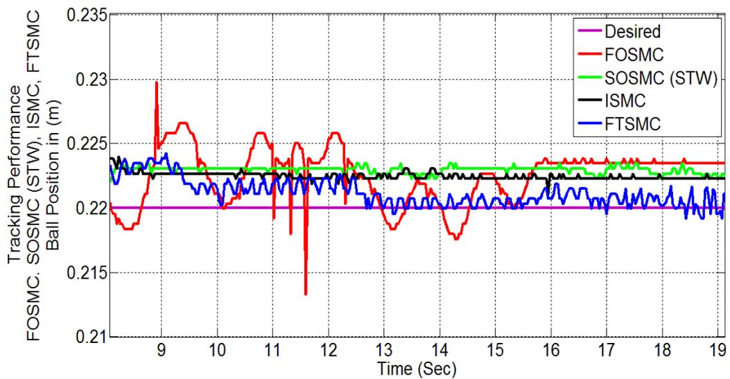
FIGURE 5.10: Zoom profile of output tracking performance of FOSMC, SOSMC(STW), ISMC and FTSMC.
