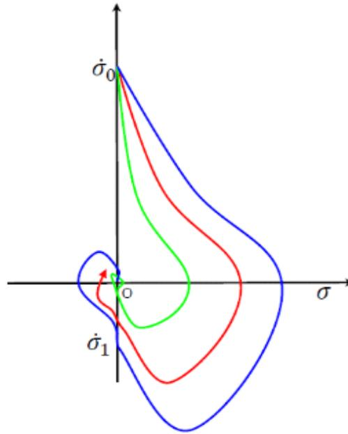
FIGURE 3.3: Phase portrait for Super Twisting Algorithm (STA) [88].
