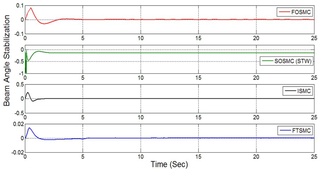
FIGURE 5.3: Separate beam angle stabilization profile of FOSMC, SOSMC(STW), ISMC and FTSMC.
