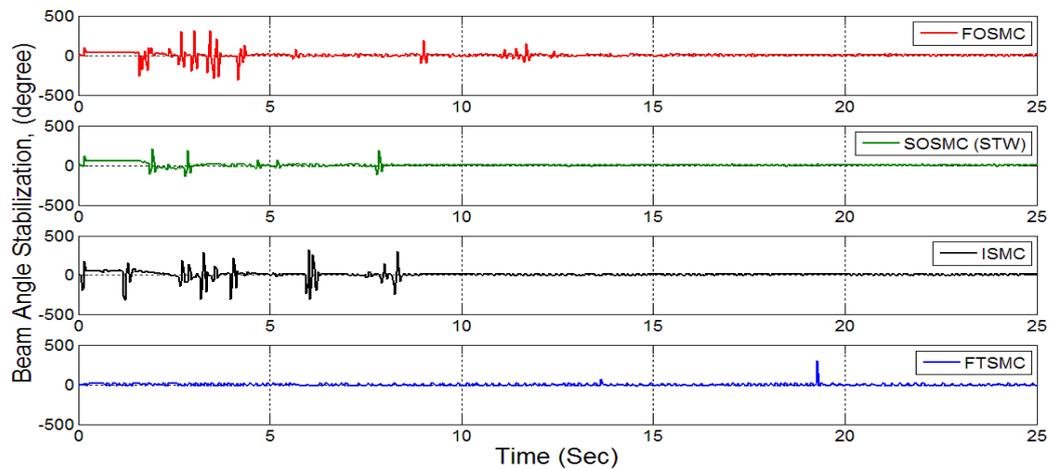
FIGURE 5.12: Separate beam angle stabilization profile of FOSMC, SOSMC(STW), ISMC and FTSMC.
