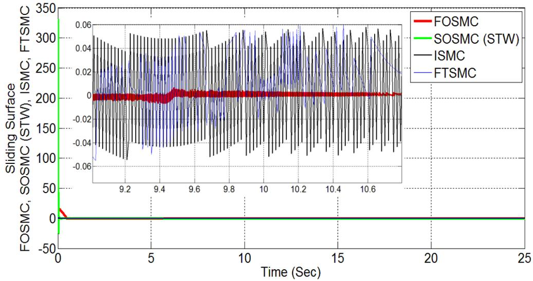
FIGURE 5.4: Sliding manifold convergence profile of FOSMC, SOSMC(STW), ISMC and FTSMC,  $r_d = 22cm$ .
