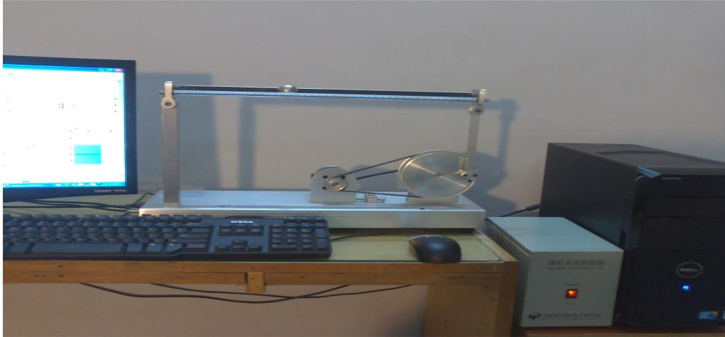
FIGURE 4.9: Experimental Setup of the Ball and Beam equipped via GoogolTech GBB1004.
