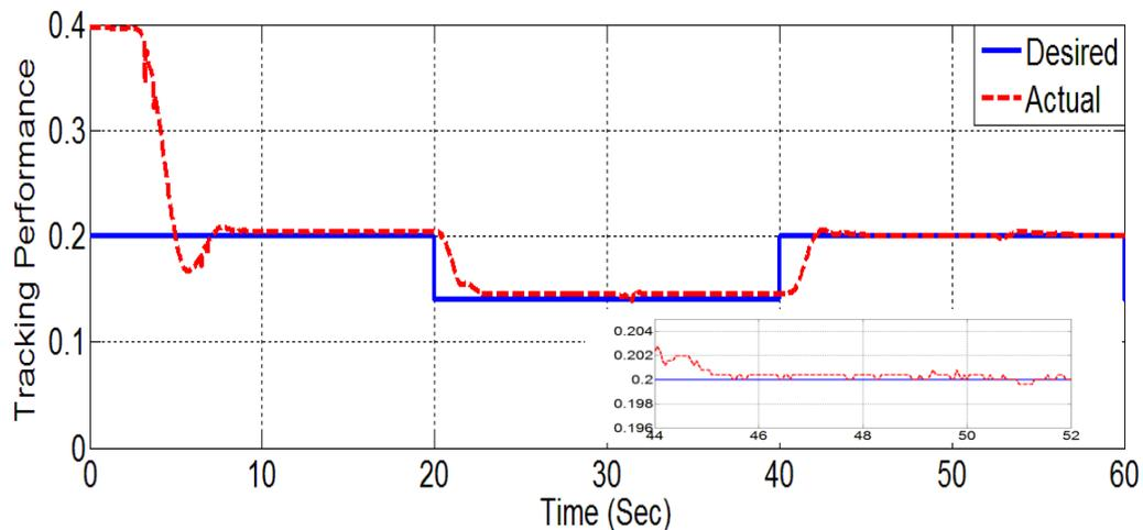
FIGURE 4.11: Output tracking performance when a square wave is used as reference/desired output.
