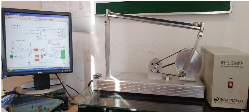
FIGURE 5.8: Experimental Setup of the Ball and Beam equipped via Googoltech GBB1004.
