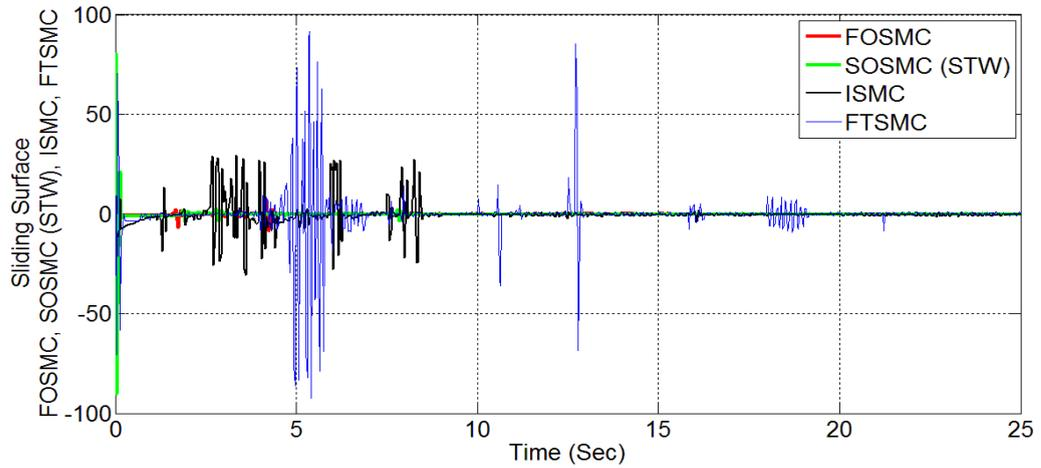
FIGURE 5.13: Sliding manifold convergence profile of FOSMC, SOSMC(STW), ISMC and FTSMC,  $r_d = 22cm$ .
