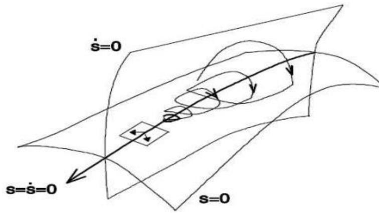
FIGURE 3.2: SOSM Control Trajectory [88].
