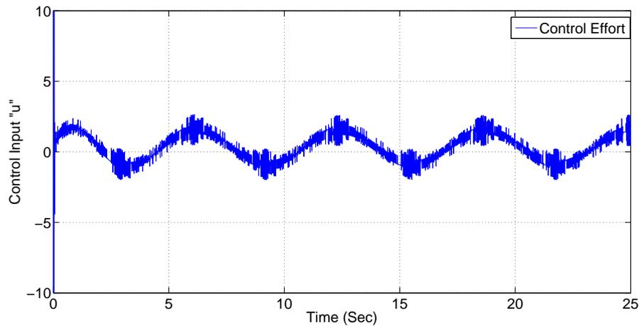
FIGURE 4.8: Control input in sinusoidal wave reference tracking.
