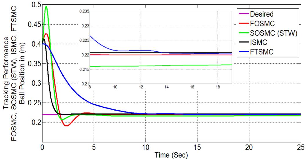
FIGURE 5.1: Output tracking performance of FOSMC, SOSMC(STW), ISMC and FTSMC,  $r_d = 22cm$ .
