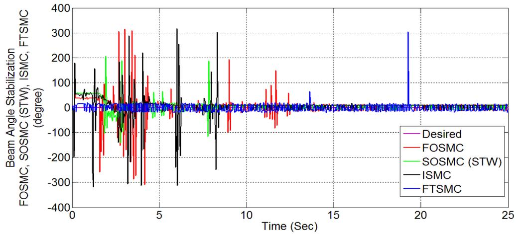
FIGURE 5.11: Beam angle stabilization profile of FOSMC, SOSMC(STW), ISMC and FTSMC,  $r_d = 22cm$ .
