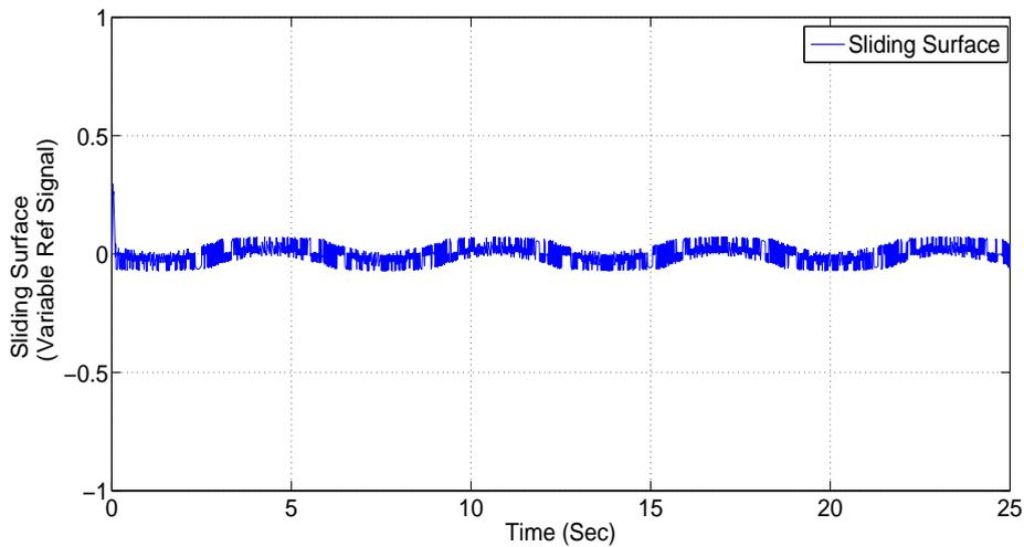
FIGURE 4.7: Sliding manifold convergence profile in case of sinusoidal wave tracking.
