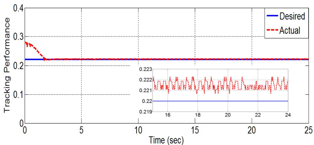
FIGURE 4.10: Output tracking performance when  $r_d = 22\text{cm}$  is set as reference/desired output.
