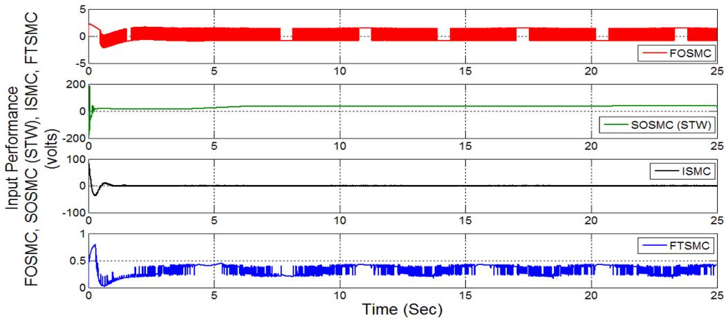
FIGURE 5.7: Separate control input profile of FOSMC, SOSMC(STW), ISMC and FTSMC.
