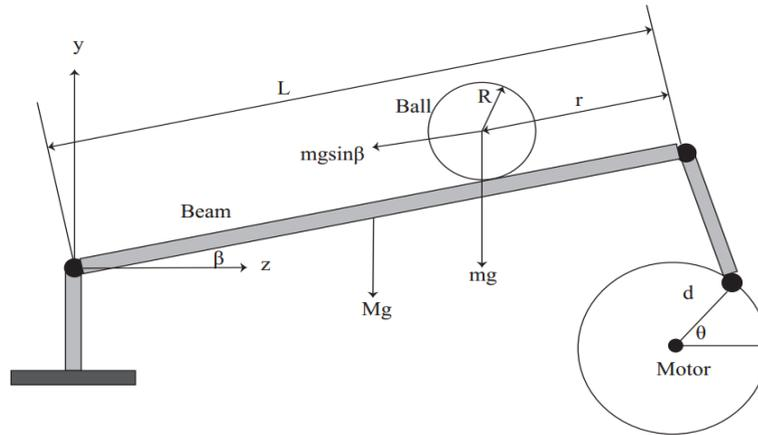
FIGURE 4.1: Schematic Diagram of the Ball and Beam System.
